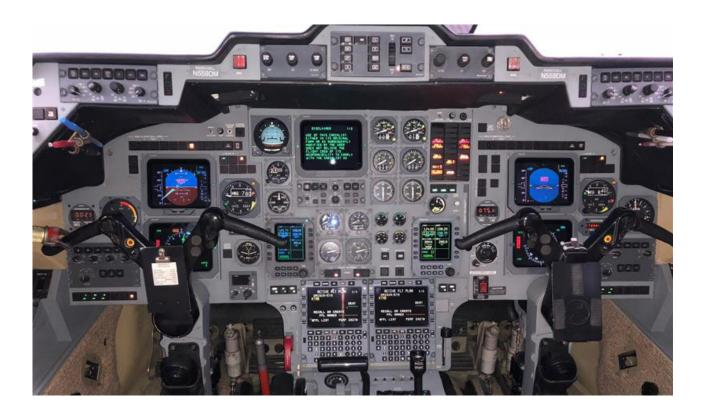
Flight System Honeywell EDZ-8000 2-Tube Transponders Autopilot Honeywell SPZ-8000 Radar Honeywell Primus 880 Comms Dual Honeywell RMZ-855 Navs Dual Honeywell RNZ-855 **Dual Honeywell**
